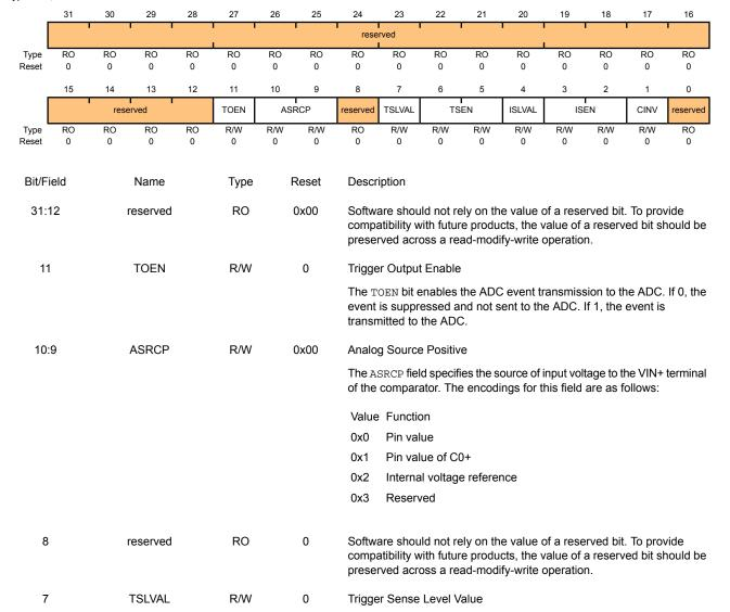
The TSLVAL bit specifies the sense value of the input that generates an ADC event if in Level Sense mode. If 0, an ADC event is generated if the comparator output is Low. Otherwise, an ADC event is generated if the comparator output is High.
