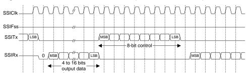
Figure 14-11. MICROWIRE Frame Format (Continuous Transfer)
