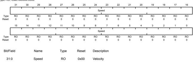
The measured speed of the quadrature encoder in pulses per period.
