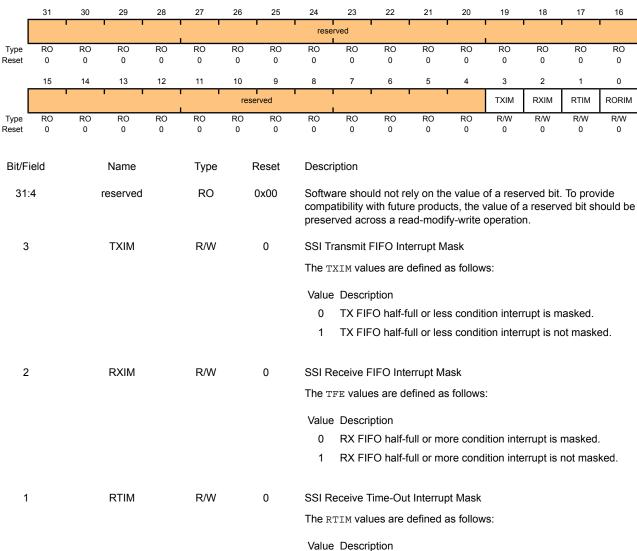
RX FIFO time-out interrupt is masked. RX FIFO time-out interrupt is not masked.
