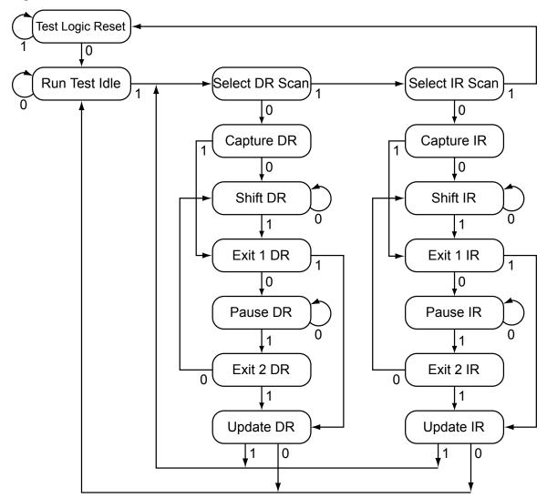
Figure 5-2. Test Access Port State Machine
