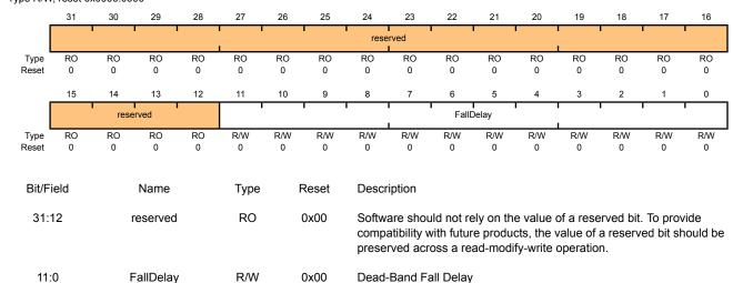
The number of clock ticks to delay the falling edge.
