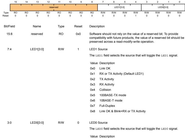
Link OK (Default LED0) 0x0 0x1 RX or TX Activity TX Activity 0x2 **RX** Activity 0x3 Collision 0x4 0x5 100BASE-TX mode 10BASE-T mode 0x6 0x7 Full-Duplex 0x8 Link OK & Blink=RX or TX Activity
