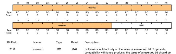
The NPR bits represent the number of packets stored in the RX FIFO. While the NPR field is greater than 0, the RXINT interrupt in the **MACRIS** register will be asserted.
