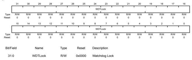
A write of the value 0x1ACC.E551 unlocks the watchdog registers for write access. A write of any other value reapplies the lock, preventing any register updates.
