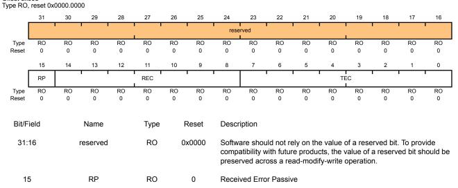
0: The Receive Error counter is below the Error Passive level (127 or less).
