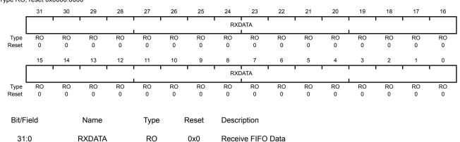
The RXDATA bits represent the next four bytes of data stored in the RX FIFO.
