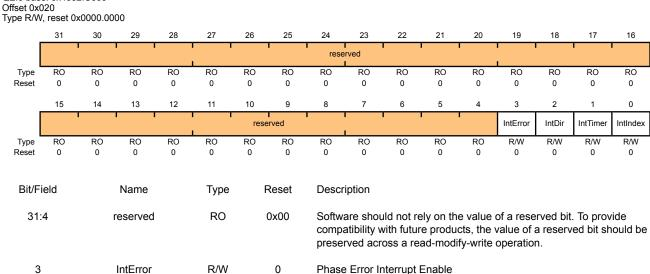
Index Pulse Detected Interrupt Enable When 1, an interrupt occurs when the index pulse is detected.
