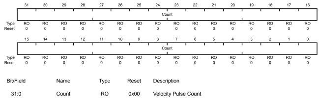
The running total of encoder pulses during this velocity timer period.
