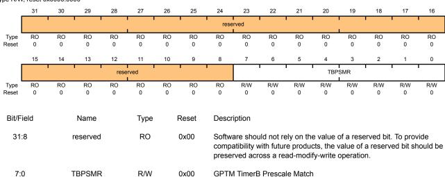
This value is used alongside **GPTMTBMATCHR** to detect timer match events while using a prescaler.
