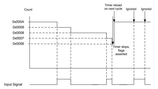
Figure 10-2. 16-Bit Input Edge Count Mode Example
