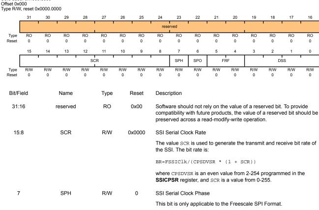
The SPH control bit selects the clock edge that captures data and allows it to change state. It has the most impact on the first bit transmitted by either allowing or not allowing a clock transition before the first data capture edge.
