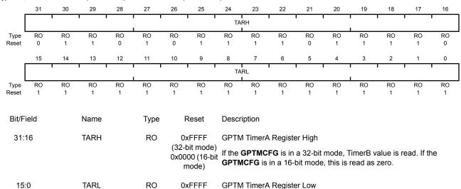
A read returns the current value of the **GPTM TimerA Count Register**, except in Input Edge Count mode, when it returns the timestamp from the last edge event.
