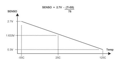
Figure 12-2. Internal Temperature Sensor Characteristic
