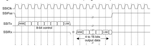
Figure 14-10. MICROWIRE Frame Format (Single Frame)
