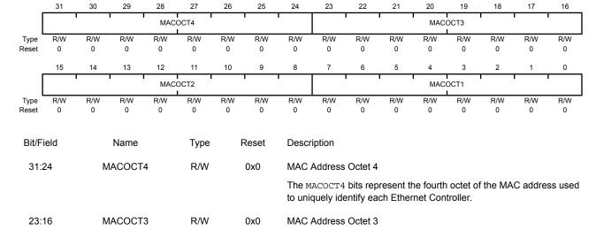
The MACOCT3 bits represent the third octet of the MAC address used to uniquely identify each Ethernet Controller.
