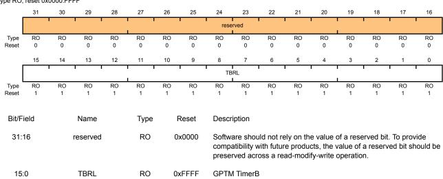
A read returns the current value of the GPTM TimerB Count Register, except in Input Edge Count mode, when it returns the timestamp from the last edge event.
