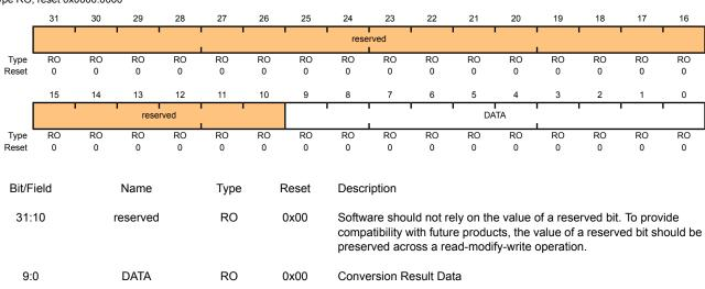
Register 17: ADC Sample Sequence FIFO 0 Status (ADCSSFSTAT0), offset 0x04C
