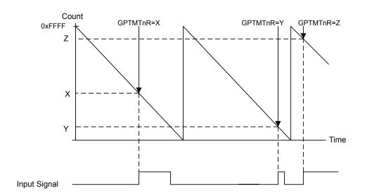
Figure 10-3. 16-Bit Input Edge Time Mode Example
