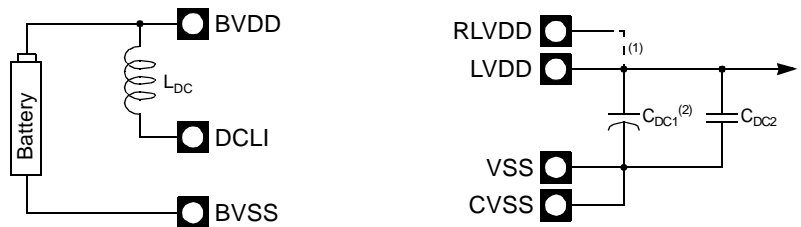
Figure 135. Battery DC-DC Connection
