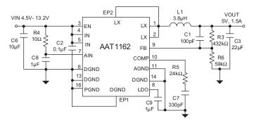
Figure 1: Typical Application Circuit.
