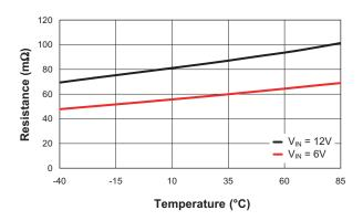
P-Channel  $R_{DS(ON)}$  vs. Temperature  $(V_{IN} = 6V)$
