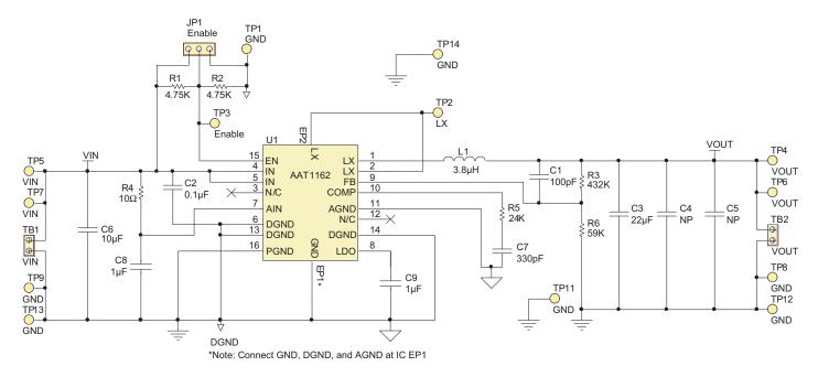
Figure 2: AAT1162 Evaluation Board Schematic.
