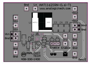
Figure 4: AAT1162 Evaluation Board Solder Side Layout.
