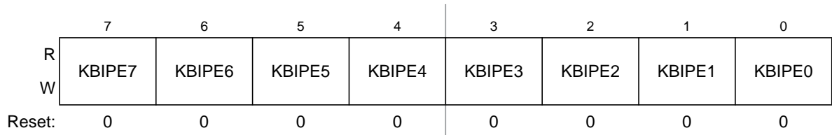
Figure 7-4. KBIx Pin Enable Register
