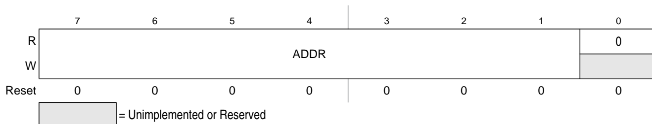
Figure 14-3. IIC Address Register (IICA)
