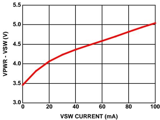
FIGURE 1. VPWR - VSW vs  $I_{VSW}$  @ AUXIN = 0V, +25°C
