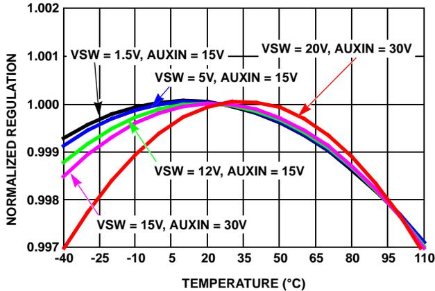
FIGURE 3. VSW REGULATION vs TEMPERATURE @
