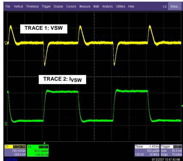
FIGURE 6. VSW TRANSIENT RESPONSE, 10mA TO 100mA STEP, VPWR = 18V, AUXIN = 15V, VSW = 12V
