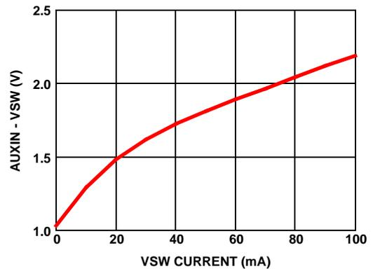
FIGURE 2. AUXIN - VSW vs  $I_{VSW}$  @ VPWR = 17V, +25°C
