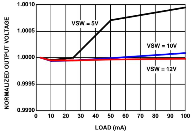
FIGURE 4. VSW REGULATION vs LOAD @ VPWR = 18V,
