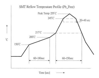
Note: 255°C is less than 20 seconds, but only pass the lead free reflow once
