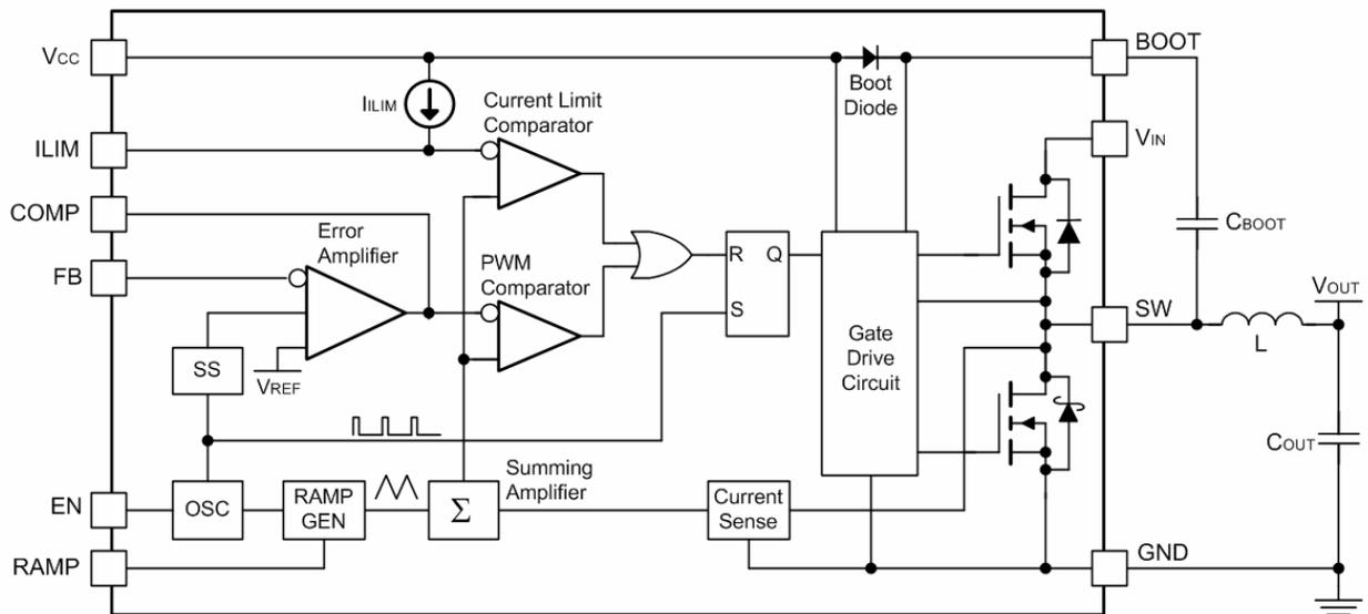
Figure 2. Block Diagram
