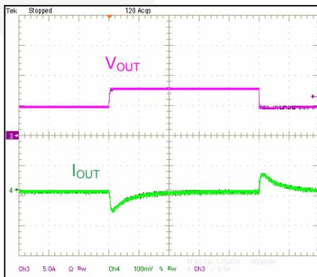
Figure 19. Transient Response, 2-8A Load
