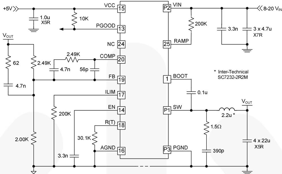
Figure 10. Application Circuit: 1.8V<sub>OUT</sub>, 500KHz
