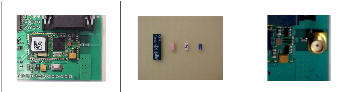
Figure 5. SMA connector for external antenna
