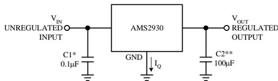
\*Required if regulator is located far from power supply filter.
