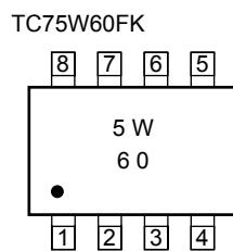
**Pin Connection (top view)**
