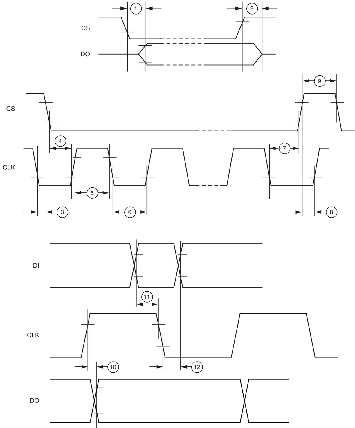
Inputs DI, CLK, CS: High level =  $0.7 \times V_{CC}$ , low level =  $0.2 \times V_{CC}$
