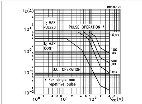
Figure 3. Derating curve
