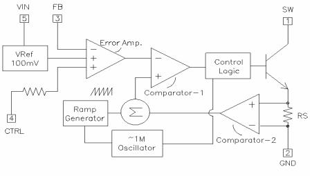
Figure 3: YB1522 Block Diagram
