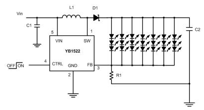
Figure 1: Typical Application Circuit
