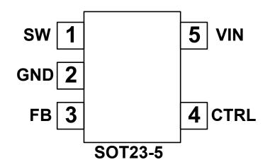
Figure 2: Pin Configuration
