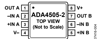
Figure 1. 8-Lead MSOP (RM-8)
