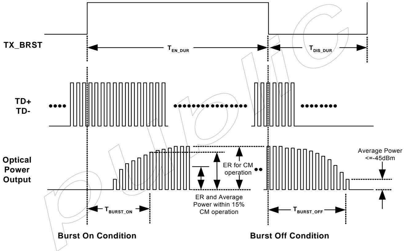
Figure 1 Timing Parameter Definition in Burst Mode Sequence
