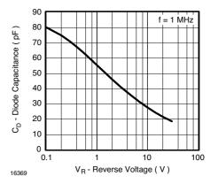
Figure 6. Diode Capacitance vs. Reverse Voltage
