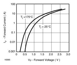
Figure 2. Forward Current vs. Forward Voltage
