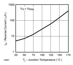
Figure 4. Reverse Current vs. Junction Temperature
