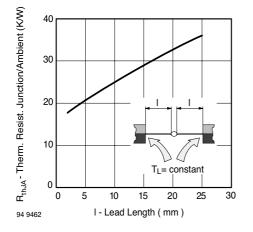
Figure 1. Max. Thermal Resistance vs. Lead Length
