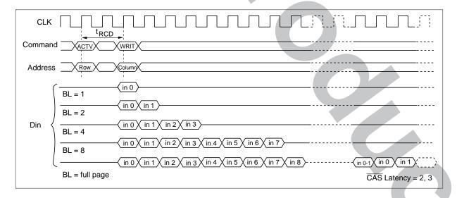
**2. Single write:** A single write operation is enabled by setting OPCODE (A9, A8) to (1, 0). In a single write operation, data is only written to the column address (AY0 to AY8; HM5212165F, AY0 to AY9; HM5212805F) and the bank select address (A12/A13) specified by the write command set cycle without regard to the burst length setting. (The latency of data input is 0 clock).
