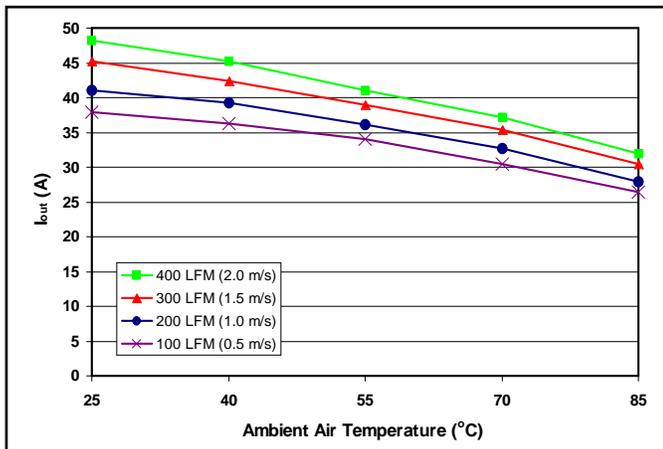
**Figure 3:** Maximum output power derating curves vs. ambient air temperature for airflow rates of 100 LFM through 400 LFM with air flowing across the converter from pin 4 to pin 1 (nominal input voltage).
