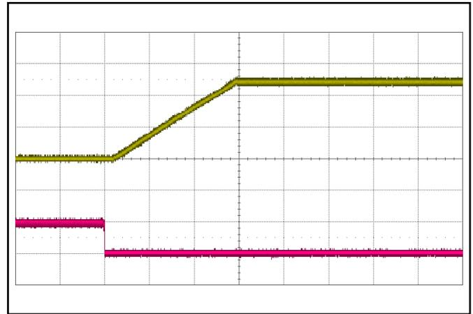
**Figure 8:** Turn-on transient at zero load (10 ms/div).
