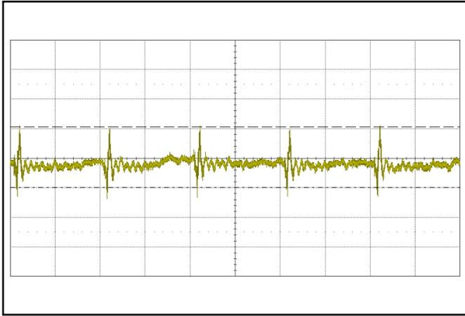
**Figure 13:** Input reflected ripple current,  $i_s$ , through a  $4.7 \mu\text{H}$  source inductor, using a  $220 \mu\text{F}$  input capacitor, at nominal input voltage and rated load current (10 mA/div;  $2 \mu\text{s}/\text{div}$ ). See Figure 11.
