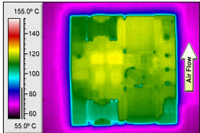
**Figure 4:** Thermal plot of converter at 36 A load current (432 W) with 55°C air flowing at the rate of 200 LFM. Air is flowing across the converter sideways from pin 4 to pin 1 (nominal input voltage).
