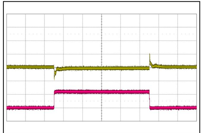
**Figure 10:** Output voltage response to step-change in load current (50%-75%-50% of  $I_{out(max)}$ ;  $dI/dt = 5 A/\mu s$ ; 1 ms/div). Load cap: 470  $\mu F$ , 15 m $\Omega$  ESR electrolytic capacitor. Top trace: Vout (500 mV/div). Bottom trace: Iout (10 A/div).
