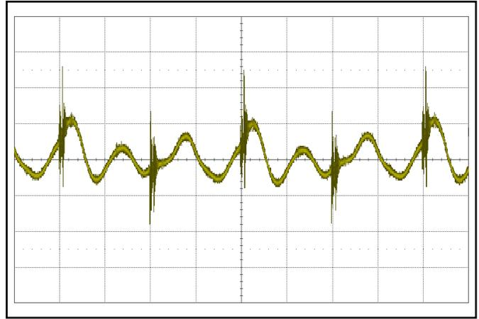
**Figure 14:** Output voltage ripple at nominal input voltage and rated load current (50 mV/div;  $2 \mu\text{s}/\text{div}$ ). Load capacitance:  $1 \mu\text{F}$  ceramic capacitor and  $15 \mu\text{F}$  tantalum capacitor. Bandwidth: 20 MHz. See Figure 11.
