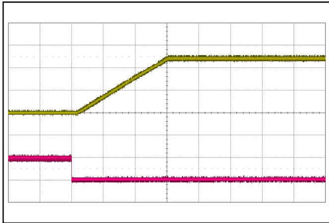
**Figure 7:** Turn-on transient at full load (resistive load) (10 ms/div).
