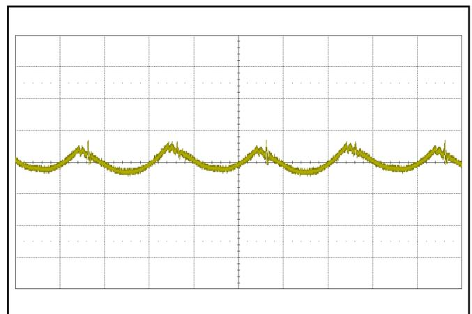
**Figure 12:** Input Terminal Ripple Current,  $i_c$ , at full rated output current and nominal input voltage with 4.7  $\mu H$  source impedance and 220  $\mu F$  electrolytic capacitor (1 A/div; 2  $\mu s$ /div). See Figure 11.
