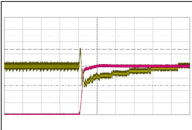
**Figure 15:** Output voltage response to step-change in input voltage (35 V to 75 V in  $300 \mu\text{s}$ ;  $1 \text{ms}/\text{div}$ ). Load cap:  $470 \mu\text{F}$ ,  $15 \text{m}\Omega$  ESR electrolytic capacitor. Top trace:  $V_{\text{out}}$  (500 mV/div). Bottom trace:  $V_{\text{in}}$  (10 V/div), at zero load current.
