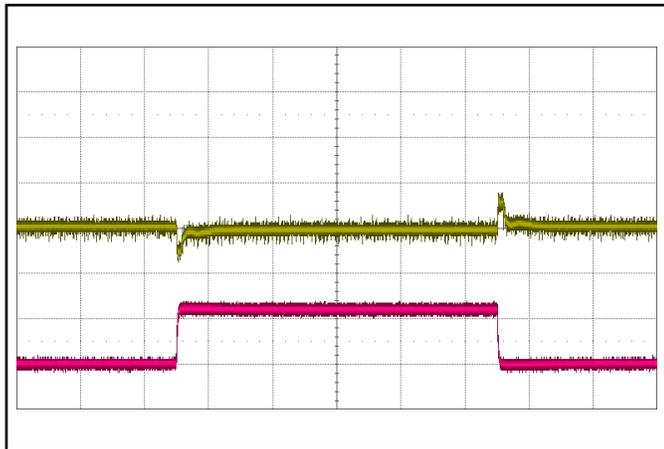
**Figure 9:** Output voltage response to step-change in load current (50%-75%-50% of  $I_{out(max)}$ ;  $dI/dt = 0.1 A/\mu s$ ; 1 ms/div). Load cap: 1  $\mu F$  ceramic and 470  $\mu F$ , 15 m $\Omega$  ESR electrolytic capacitors. Top trace: Vout (500 mV/div). Bottom trace: Iout (10 A/div).
