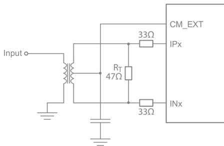
Figure 4. Transformer-Coupled Input
