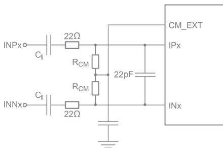
Figure 5. AC-Coupled Input
