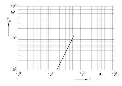
Ohmic power dissipation  $P_{\text{\scriptsize R}}$  vs. RMS current value I
