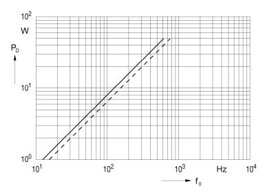
Dielectric power dissipation  $P_D$  vs. repetition frequency  $f_0$
