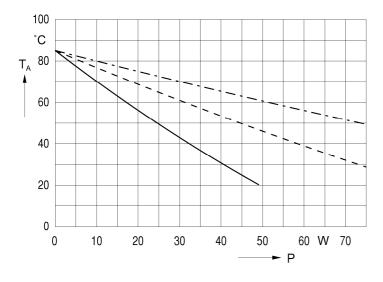
Permissible ambient temperature  $T_{\text{\tiny A}}$  vs. total power dissipation P
