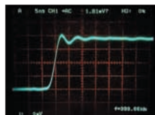
Input: 100 mA-p-p (Oscilloscope bandwidth 400 MHz)
