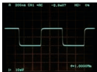
Input: 1 MHz square wave 200 mA-p-p (Oscilloscope bandwidth 400 MHz)
