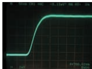
Input: 1 Ap-p (Oscilloscope bandwidth 20 MHz)
