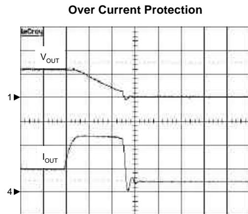
$C_{OUT}=10\mu F$ ,  $C_{IN}=10\mu F$ ,  $I_{OUT}=1A$  to  $2.3A$
