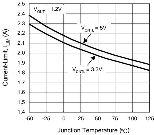
Short Current-Limit vs. Junction Temperature
