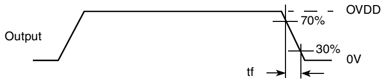
Figure 7. Definition of Timing for Standard- and Fast-Mode
