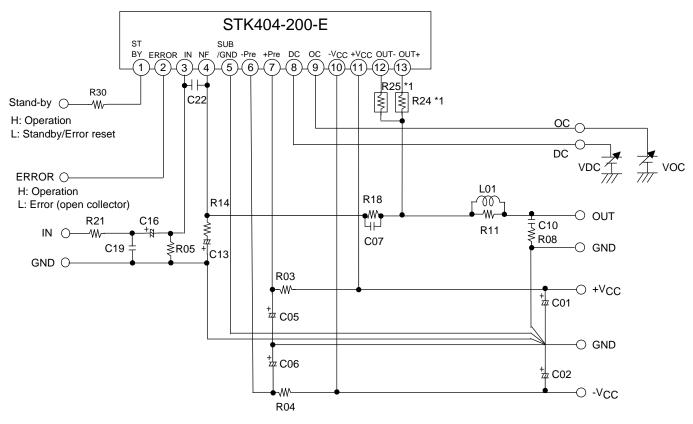
\*1 Metal plate cement resistor:  $0.22\Omega \pm 10\%$  (5W)
