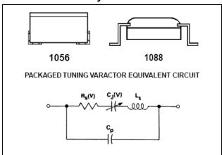
The MA46H070 through MA46H073 (gamma 0.75) family of constant gamma hyperabrupt GaAs tuning varactors has quality factor approaching that of abrupt junction varactors, but higher capacitance change versus tuning voltage. These diodes are very well suited for narrowerbandwidth VCOs and VTFs where wide tuning range and very high quality factor are required.
