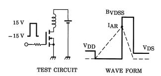
$$\begin{aligned} R_G &= 25~\Omega \\ V_{DD} &= 25~V,~L = 840~\mu H \end{aligned} \qquad EAS &= \frac{1}{2} \cdot L \cdot I^2 \cdot \left( \frac{BVDSS}{BVDSS - VDD} \right) \end{aligned}$$
