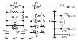
X1:5.08-mm-pitch 2-pin oscillator X2:2.54-mm-pitch 2-pin oscillator X3:2.54-mm-pitch 3-pin oscillator
