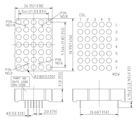
NOTES: 1. All dimensions are in millimeters. Tolerances are  $\pm$  0.25 mm unless otherwise note.
