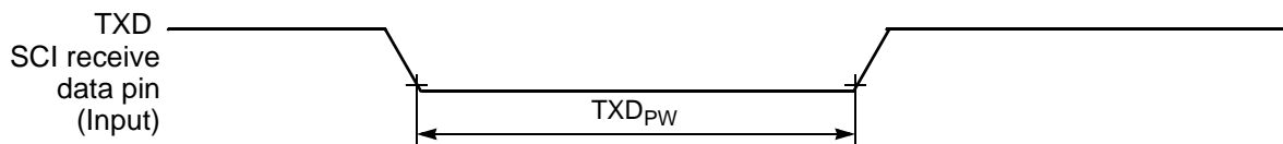
Figure 10-13 TXD Pulse Width
