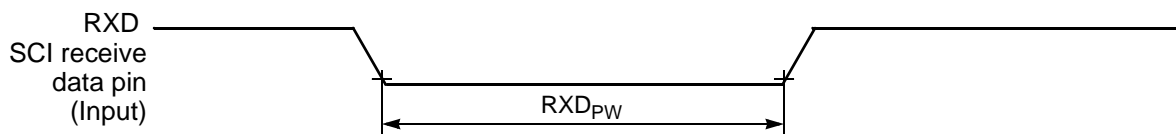
Figure 10-12 RXD Pulse Width
