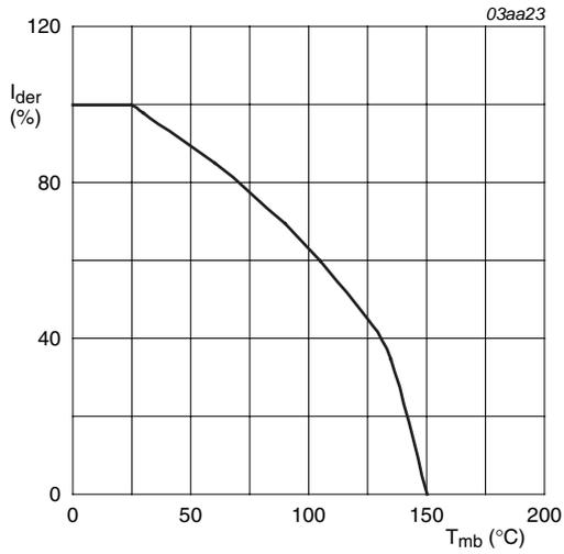
$$I_{der} = \frac{I_D}{I_{D(25^\circ\text{C})}} \times 100\%$$
