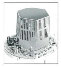
Unipolar ionization chamber provides stable response to a broad range of fires!
