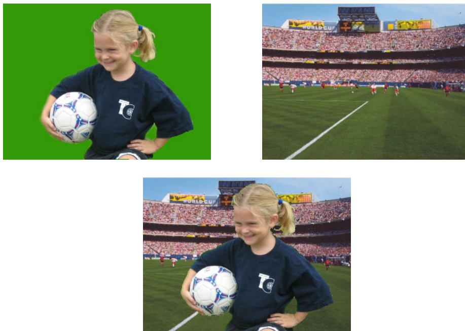
Figure 17-13. Pixel Pipeline (PXP) Colorkey Example
