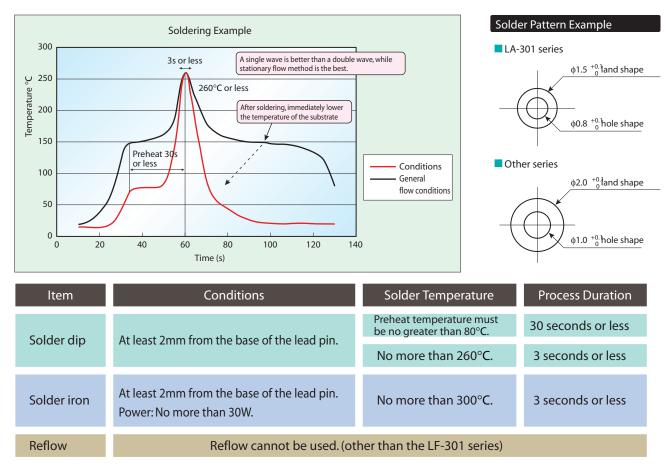
\*Please use a resin-based flux, since flux that is acidic or highly alkaline could cause corrosion.
