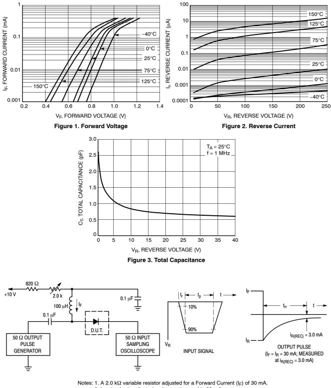
2. Input pulse is adjusted so  $I_{R(peak)}$  is equal to 30 mA.
