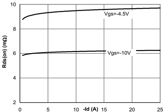
Figure 3: On-Resistance vs. Drain Current and Gate Voltage
