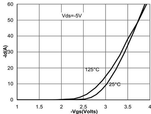
Figure 2: Transfer Characteristics
