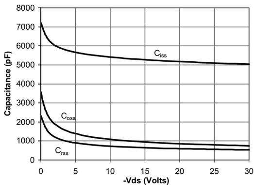
Figure 8: Capacitance Characteristics
