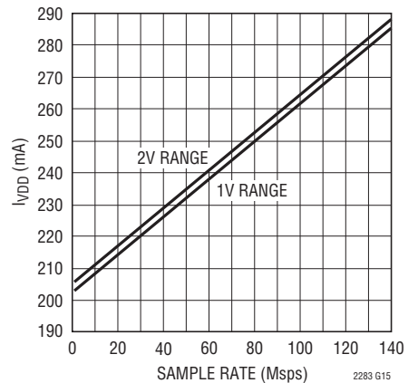
I_{VDD} vs Sample Rate, 5MHz Sine Wave Input, -1dB
