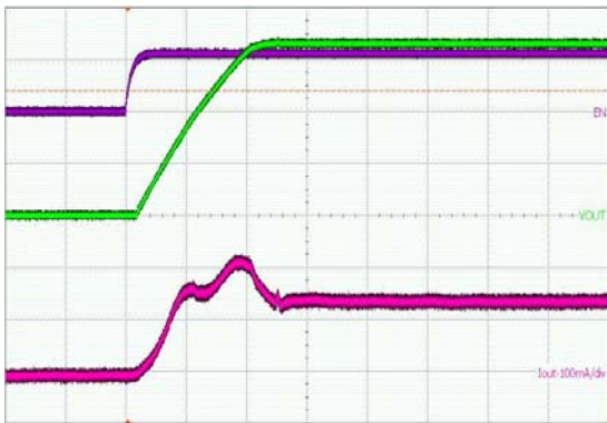
( V_{IN} = 5\text{ V} , I_{LOAD} = 100\text{ mA} , L = 3.3\text{ }\mu\text{H} , C_{OUT} = 2 \times 22\text{ }\mu\text{F} ) Upper Trace: EN Pin Voltage, 2 V/div Middle Trace: Output Voltage, 1 V/div Lower Trace: Inductor Current, 100 mA/div
