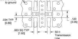
Dimensions are in Inches [Millimeters] JP506 Rev A Mounting Footprint
