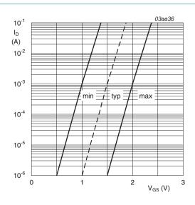
$T_j = 25 \,^{\circ}C; V_{DS} = V_{GS}$
