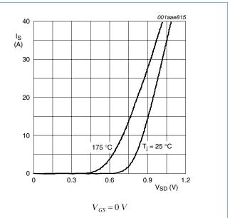
Fig 14. Source current as a function of source-drain voltage; typical values
