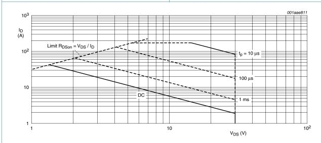
$T_{mb}$  = 25 °C;  $I_{DM}$  is single pulse;  $V_{GS}$  = 10 V
