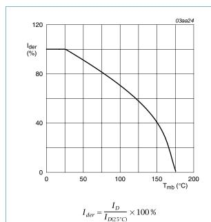
Normalized continuous drain current as a Fig 1. function of mounting base temperature
