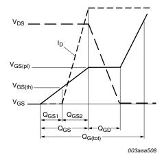
Fig 12. Gate charge waveform definitions
