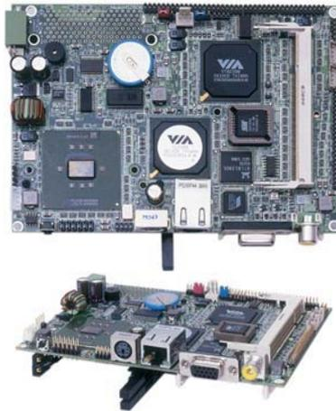
The HS-2606 is a 100/133MHz FSB VIA CLE266/VT8235 chipset-based board designed for Mini PCI Local Bus ULV Intel® Celeron® processor 400/650MHz. These features combine and make the HS-2606 an ideal all-in-one industrial single board computer. Additional features include an enhanced I/O with CF, PCMCIA, CRT/Panel, audio, LAN TV-Out, 4 COM, and USB2.0 interfaces.
