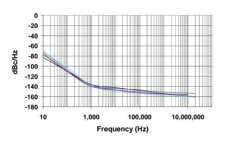
Typical phase noise plot for 5 oscillators at different output frequencies.
