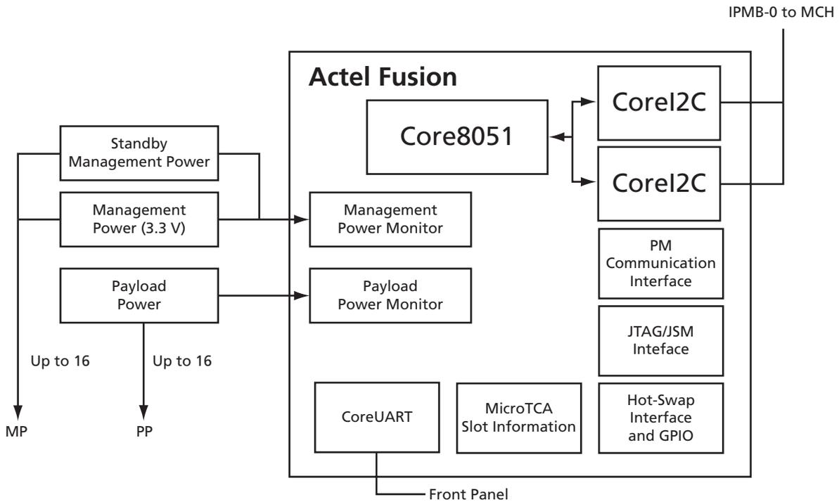
Figure 2 • Power Module Fusion Device Block Diagram
