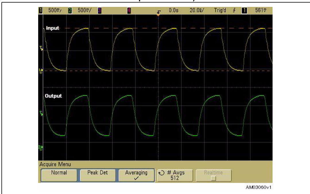
Figure 32. Sine wave input clock vs. output clock (STCD1040, 1.8 V version, 26 MHz sine wave master clock input from TCXO)
