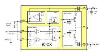
Figure 4: Configuration as high side
