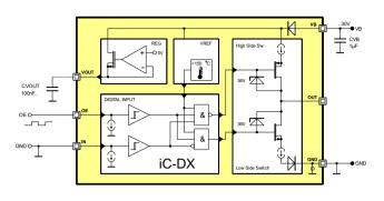
Figure 5: Configuration as low side
