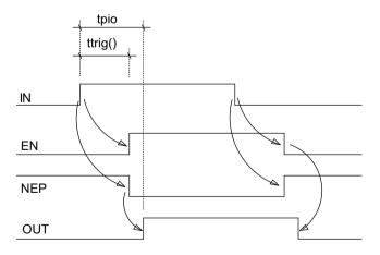
Figure 7: Timing diagram in push-pull operation mode
