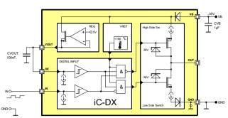
Figure 6: Configuration as Pushpull
