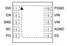
2.5mm x 2.5mm Thin MLF<sup>®</sup> (MT) Fixed Output Voltage (Top View)
