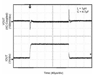
Line Transient (3.6V to 5.5V @ 20mA Load)
