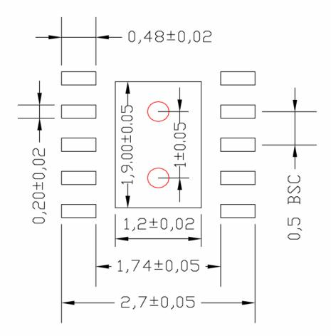
Red circle indicates Thermal Via. Size should be .300-.350 mm in diameter and it should be connected to GND plane for maximum thermal performance.
