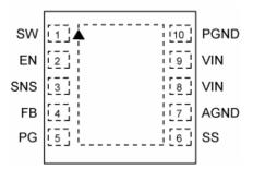
2.5mm x 2.5mm Thin MLF<sup>®</sup> (MT) Adjustable Output Voltage (Top View)
