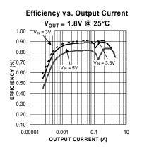
Figure 2. Efficiency Under Load
