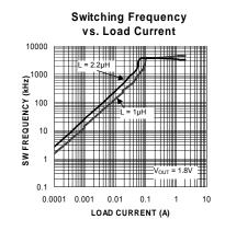
Figure 3. SW Frequency vs. Output Current
