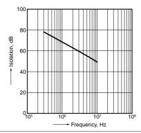
15. Insertion loss vs. frequency characteristics (50 $\Omega$  impedance) Measured portion: between terminals 3 and 4
