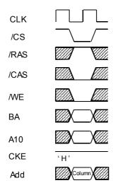
If the mode register is in the burst write mode, this command sets the burst start address given by the column address to begin the burst write operation. The first write data in burst mode can input with this command with subsequent data on following clicks.
