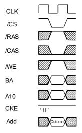
Read data is available after /CAS latency requirements have been met. This command sets the burst start address given by the column.
