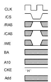
This command can stop the current burst operation.
