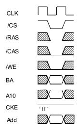
The EM488M3244VBA have a mode register that defines how the device operates. In this command, A0 through BA are the data input pins. After power on, the mode register set command must be executed to initialize the device. The mode register can be set only when all banks are in idle state. The EM488M3244VBA, cannot accept any other commands, only during 2CLK can following this command.
