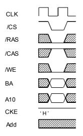
This command begins precharge operation of the bank selected by. When A10 is high,all banks are precharged, regardless of. When A10 is low,only the bank selected by BA is precharged.
