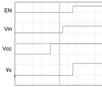
Fig.2 Input Voltage Sequence
