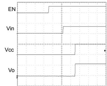
Fig.6 Input Voltage Sequence
