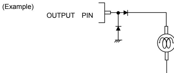
9. We are certain that examples of applied circuit diagrams are recommendable, but you are requested to thoroughly confirm the characteristics before using the IC. In addition, when the IC is used with the external circuit changed, decide the IC with sufficient margin provided while consideration is being given not only to static characteristics but also variations of external parts and our IC including transient characteristics.
