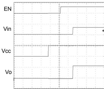
Fig.4 Input Voltage Sequence
