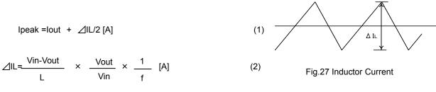
(  $\eta$  : Efficiency,  $\angle$ IL : Output Ripple Current, f : Switching Frequency )
