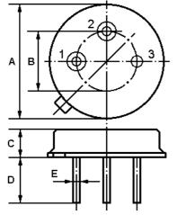
Pin Configuration 1 Input / Output 2 Output / Input 3 Case Ground Dimension Data (unit: mm) А 9.30±0.20 В 5.08±0.10 С 3.40±0.20 3±0.20 / 5±0.20 D Е 0.45±0.20
